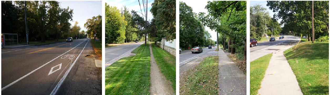
*Field photos of a dedicated cycle lane and variations on pedestrian connectivity – from an informal path on the boulevard to a sidewalk setback from roadway edge to a sidewalk transitioning to the street edge*
